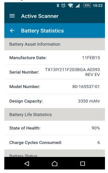
Figure 1-18 Advanced Tab - Battery Statistics
