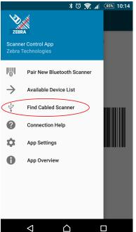
**d.** Select **Find Cabled Scanner** from the menu to display the SNAPI bar code.
