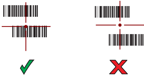
Figure 4-4 Pick List Mode with Multiple Bar Codes in Aiming Pattern
